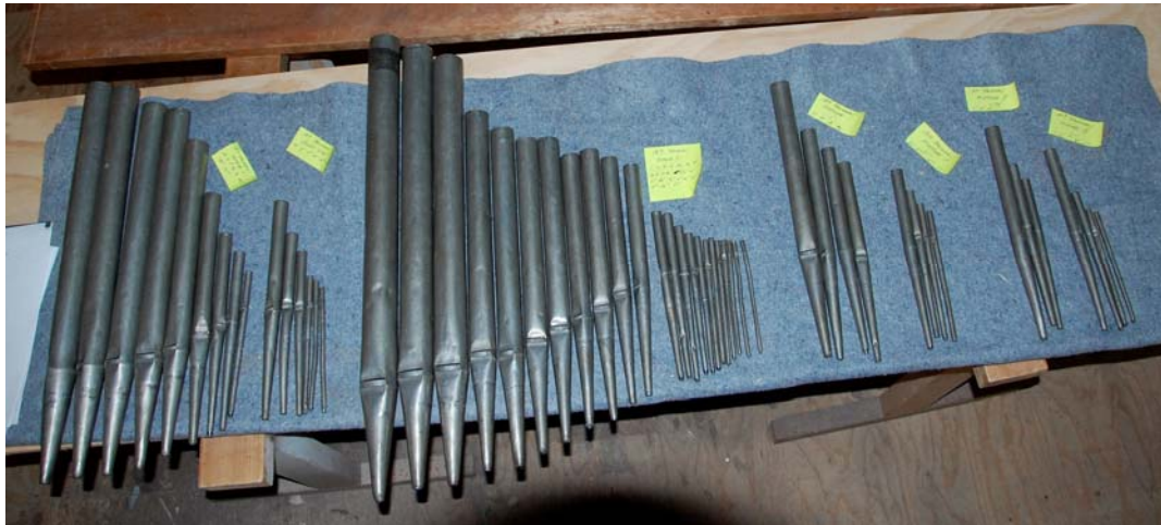
Original Bachman organ pipes belonging to the Octav 4'; Quinte 2 2/3'; Octav 2'; and Mixture
